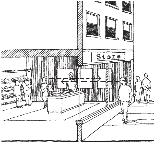
Fig. B.5.d 1 & 2: Ground-level transparency must provide visibility into and from the interior use.
