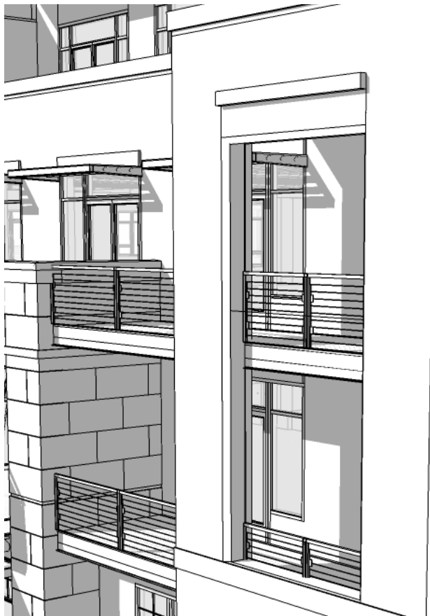
Fig. B.2.d.10 (2): Wall planes over 750 square feet are divided into distinct planes by incorporating porches and/or extending an architectural bay.
