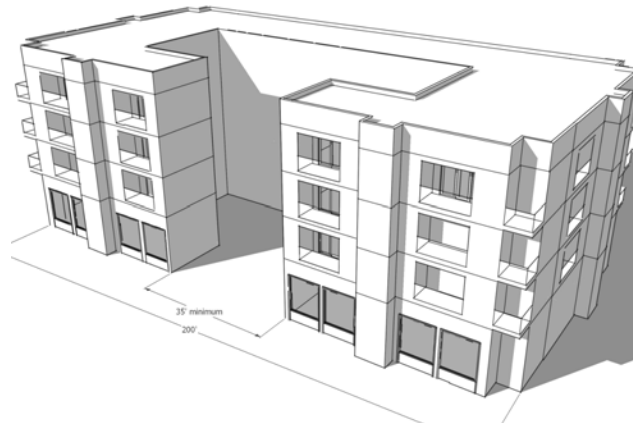
Fig. B.1.d.9: Structures facing a street can increase horizontal length to 200 feet by providing an internal courtyard with a minimum 35-foot width.
