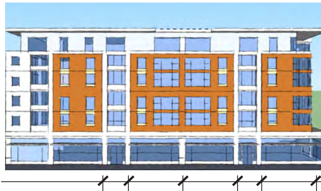
Fig. B.2.c.4: Belt line above the ground level and regular cadence of bays and storefronts.
