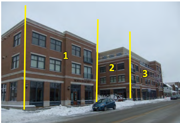
Fig B.1.d.1: A building with a large footprint is divided into multiple masses, each greater than 25% of the footprint.
