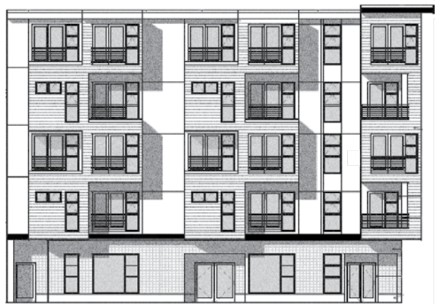
Fig. B.2.d.12. Elevation indicates minimum glazing percentages of 40% at ground floor and 40% at upper floors.
