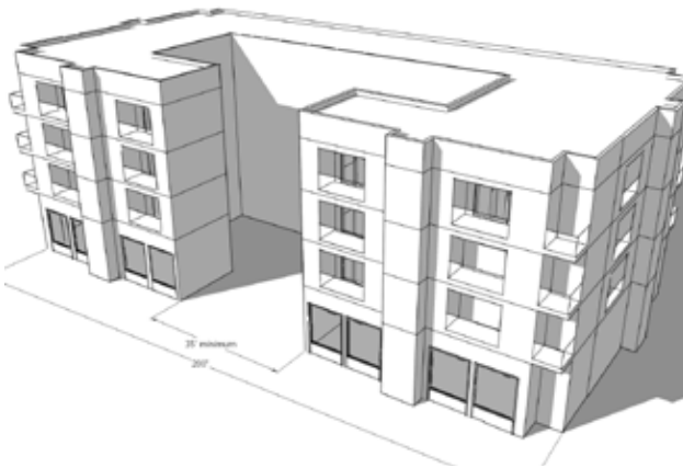
Fig. B.1.d.2. Structures facing a street can increase horizontal length to 200' by providing an internal courtyard with a minimum 35' foot width.
