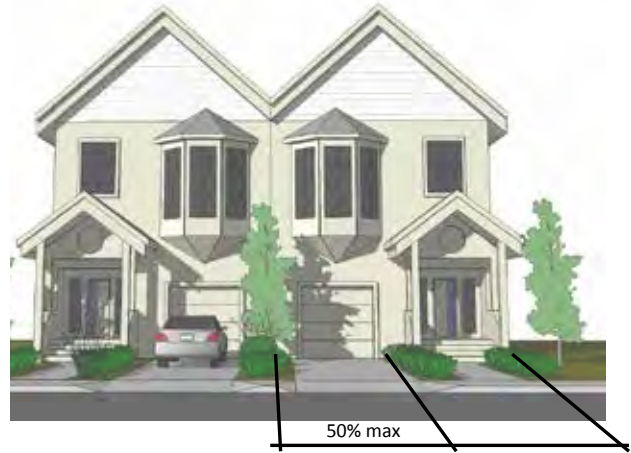
Fig. A.1.d.7. Street-facing garages associated with duplexes and multi-family townhouses shall have a maximum width of fifty percent (50%) of the overall building width.
