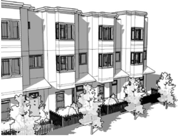
Fig. B.1.d.1. Exterior wall offsets shall reflect the living unit modules when individual unit entries face the street.
