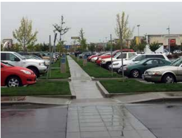
Fig. A.8.D.6: A pedestrian circulation route which is separated from parking stalls with curbs, landscaping and illuminated bollards.
