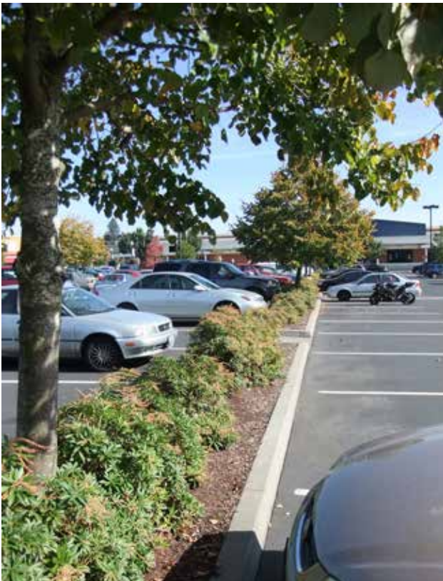
Fig. A.7.D.5.B.1: Landscaped row visually divides the parking areas while potentially providing space for stormwater management.
