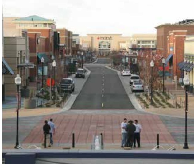
Fig. A.2.C.2: Landscaping, street trees and pedestrian-scaled lighting enhance the pedestrian areas on internal streets and primary internal drives.
