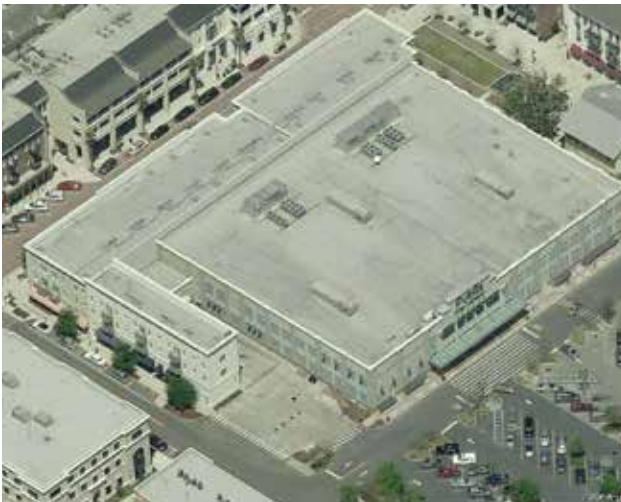
Fig. A.10.D.1.E: Aerial view of a building which use liner spaces to conceal service and loading areas.
