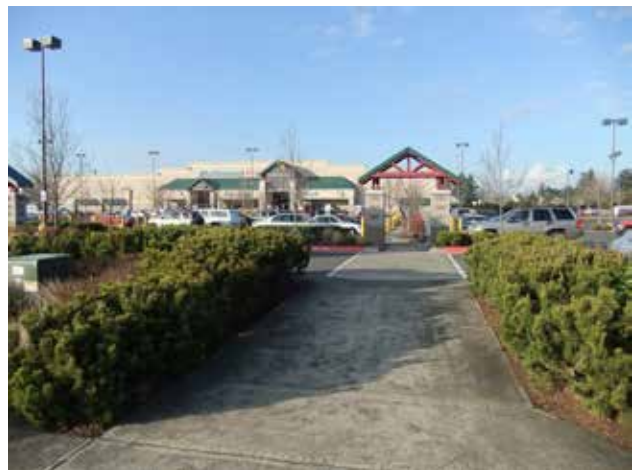
Fig. A.8.C.1(2): An internal pedestrian circulation route which connects to a public street.
