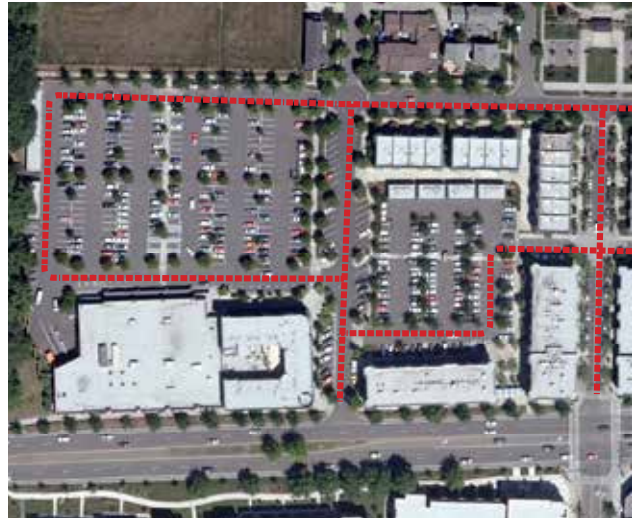
Fig. A.1.D.4: Many vehicular and pedestrian connections are preset between adjacent commercial uses and sites.
