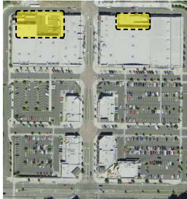
Fig. A.10.C.1: Service areas located away from public areas of the site.
