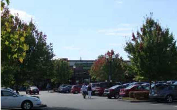
Fig. A.7.D.5: Internal parking landscaping visually reduces the scale of the parking area and shades hardscapes to reduce heat islands.
